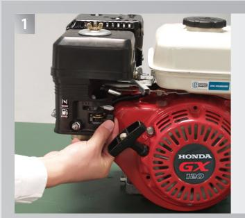
Turn the fuel valve lever to the ON position.
