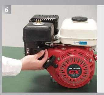
Gradually move the choke lever to the OPEN position as the engine warms up.
