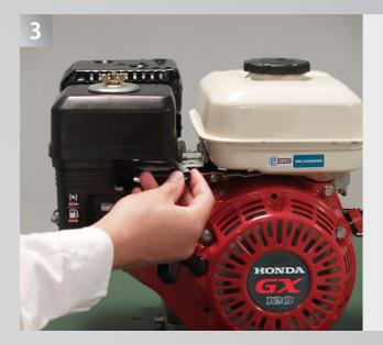
Move the throttle control lever slightly to the left.
