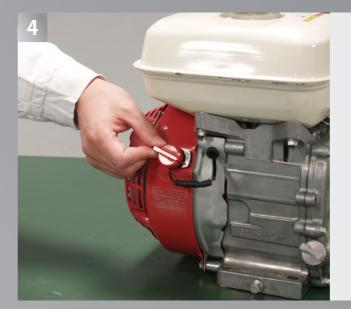
Turn the engine switch to the ON position.
