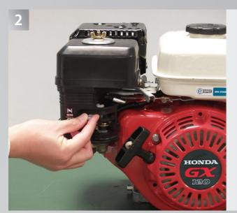
Move the choke lever to the CLOSED position.
